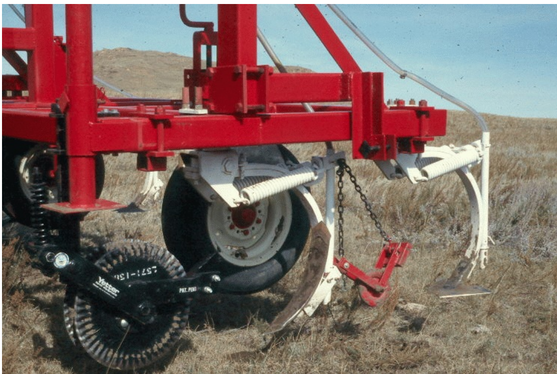
Fig. 2. Interseeding tools: double straight coulters, 3-inch twisted chisel plow shovel, and 12- inch cultivator sweep with tip removed.
