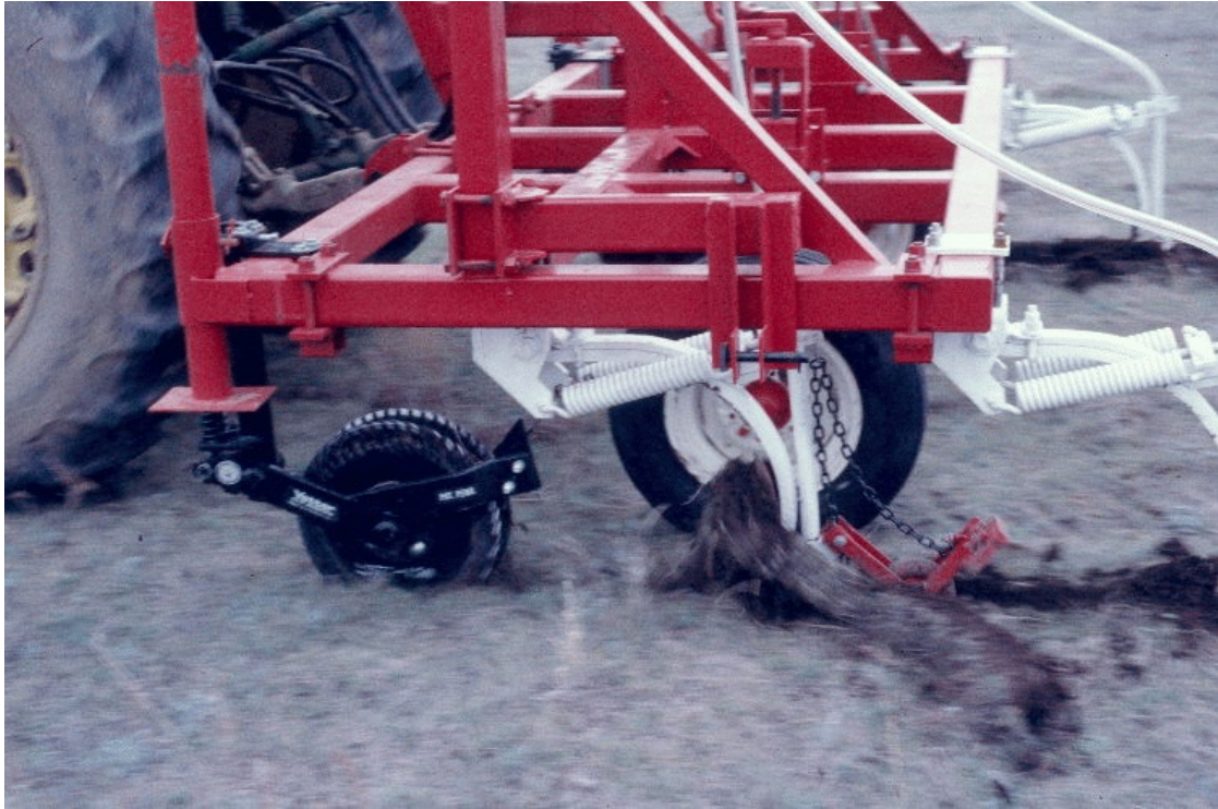
Fig. 3. Interseeding alfalfa into grassland with triple-toolbar machine.
