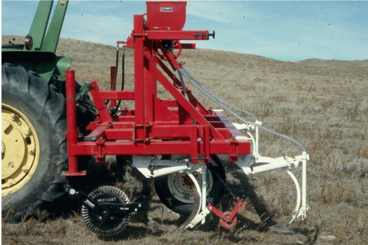
Triple-toolbar interseeding machine with double straight coulters, three-inch twisted chisel plow shovel, and twelve-inch cultivator sweep with tip removed.
