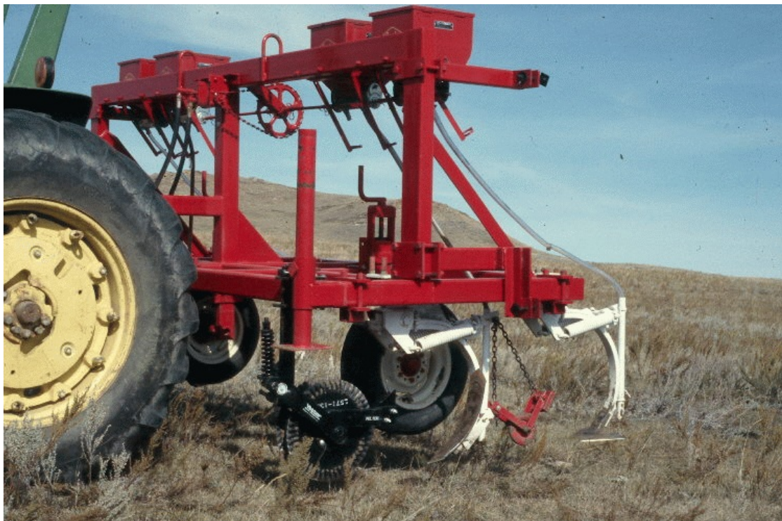
Fig. 1. Triple-toolbar interseeding machine.
